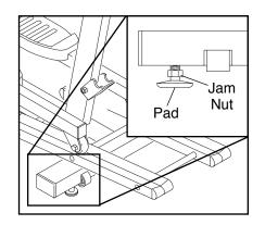
leveling pads as needed until the elliptical crosstrainer is level. When the leveling pads are properly adjusted, firmly retighten the jam nuts.
